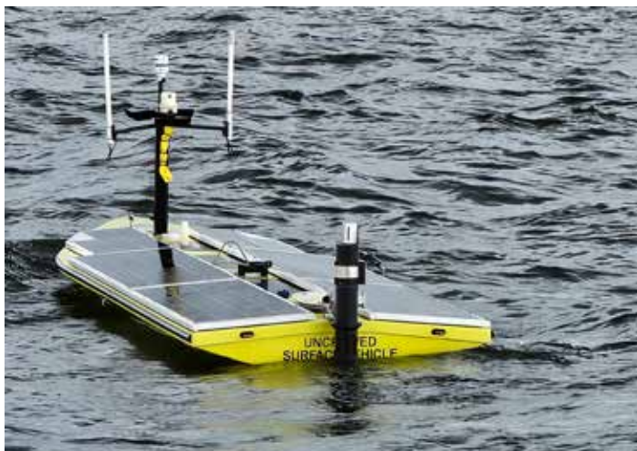
Figure 3: The Endura-3 deployed on SeaTrac's SP-48 USV. In partnership with the University of Southern Mississippi (USM), SeaTrac conducted a fourteen-day mission to analyze potential hypoxia levels and their impact on marine life in the US Gulf Coast. We asked James, the lead from USM about the impact of the Endura-3: he said, “this simplifies everything.”
