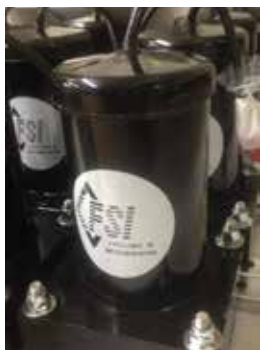
A high power 1-10KHz transducer
